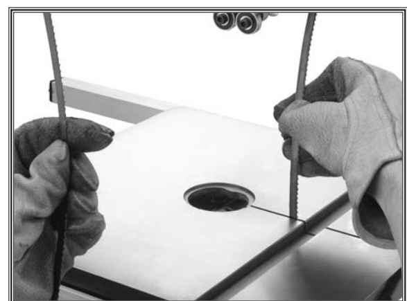
Figure 51. Changing the blade.
